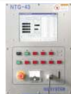
User friendly 4 axis CNC for tool grinder
